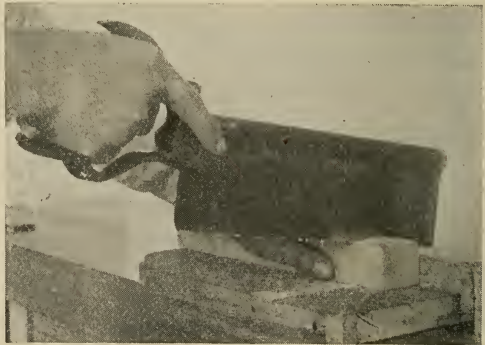
Fig. 71 - Sawing, Third Position
